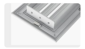
In the magnet system cod. M/01 it is necessary to associate a counterframe to the grille/nozzle (for example a FITT Agix ® counterframe of the series - C/01) or a section of galvanized channel ending with a border or even a series of L-shaped corners in galvanized sheet metal that can be fixed to the plenum/adapter (brackets, provided by the customer) in a number equal to the number of magnets.
